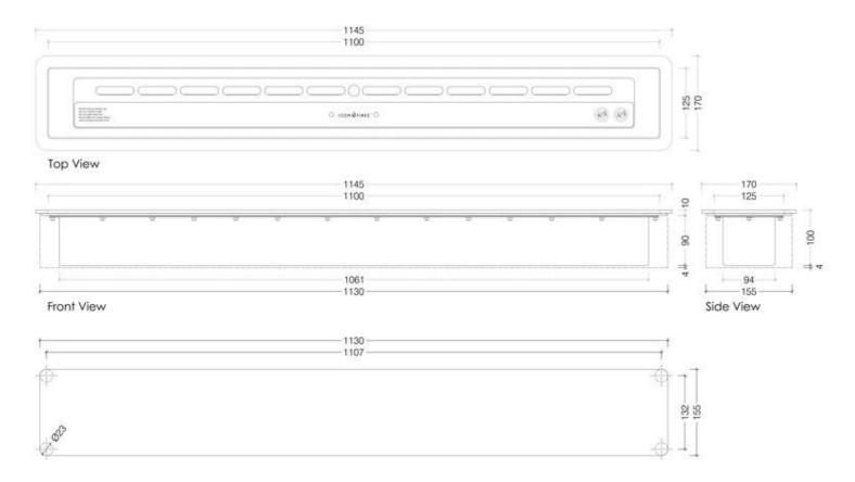
Slimline 1100 Biofuel Burner With Mount Plate
